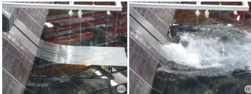
Figure 2. Physical model test in 3D with (a) initial conditions and (b) tsunami generation and propagation at t \approx 0.7 s.
