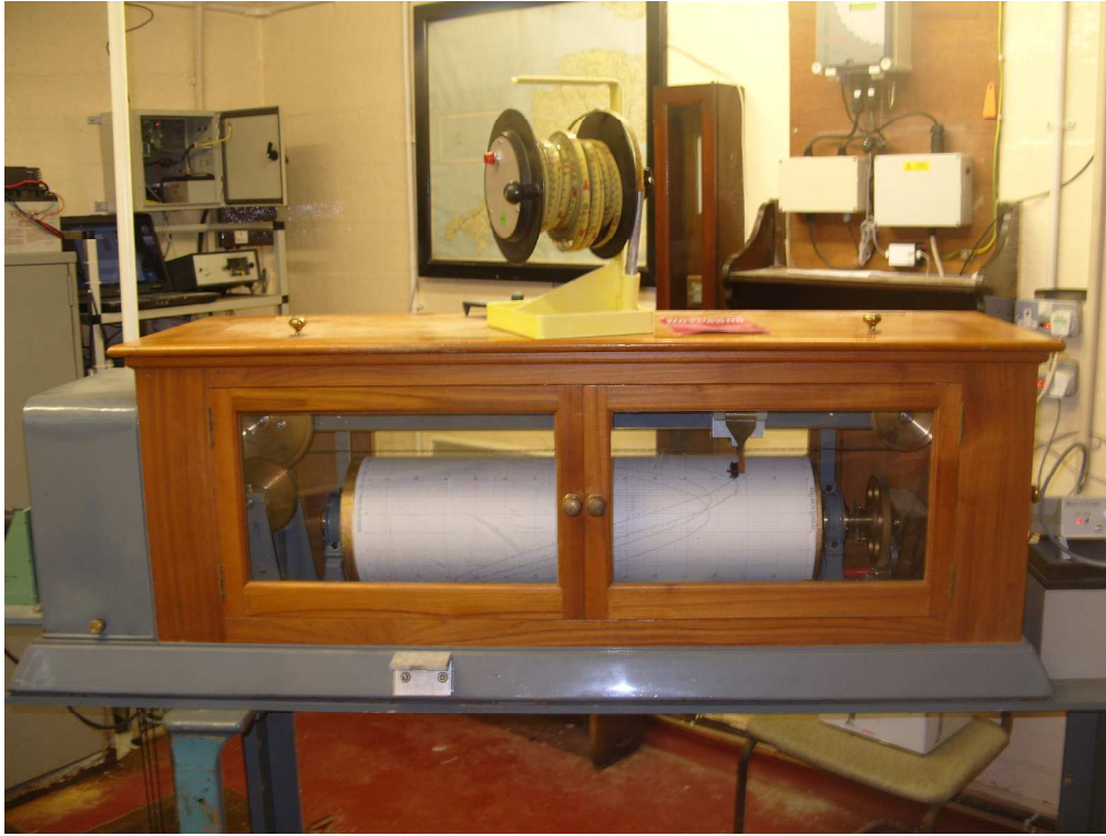
Figure 7. The Munro tide gauge installed in 1983 and located above the stilling well. The white L-piece on the front of its frame is the Contact Point from which dipping measurements are made in order to confirm that the gauge is recording to the correct datum. The dipper itself is shown on top of the gauge. (Photograph Les Bradley). 965x723mm (96 x 96 DPI)
