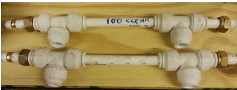
220 221 A: PHFHE heat exchanger (fibre number: 100 and 200)
