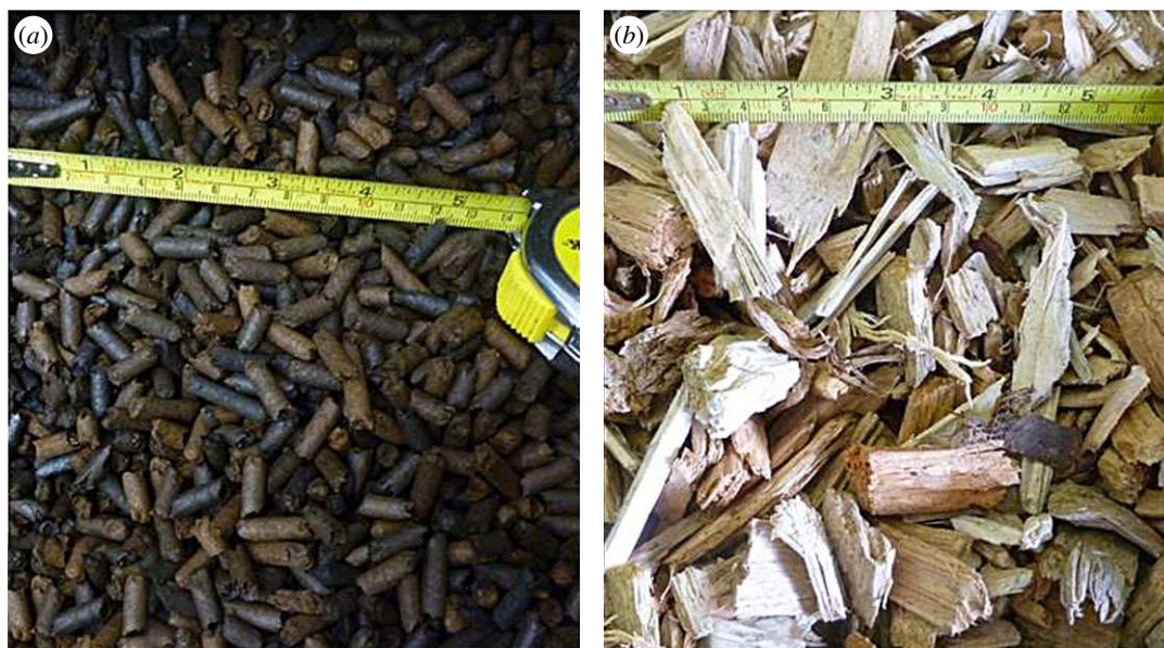
Figure 1. (a) Torrefied pellet and (b) P45 mixed wood chip used for gasification.
