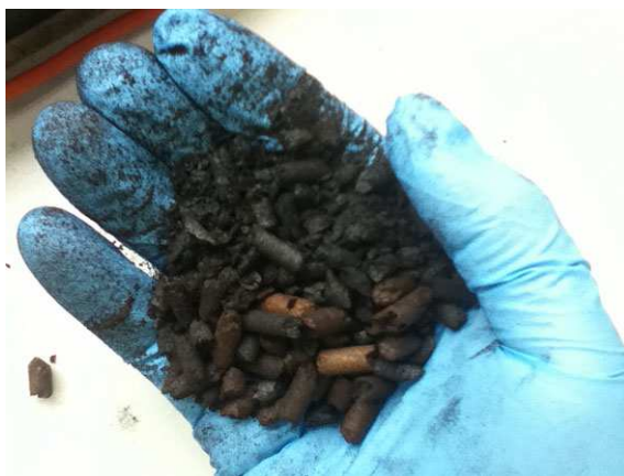
Figure 7. Torrefied pellet extracted from the combustion zone of Power Pallet gasifier after failed experimental run.
