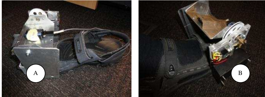
Figure 2 RIMU prototype with (left) IMU mounted on a rotating platform, and (right) the RIMU controller.
