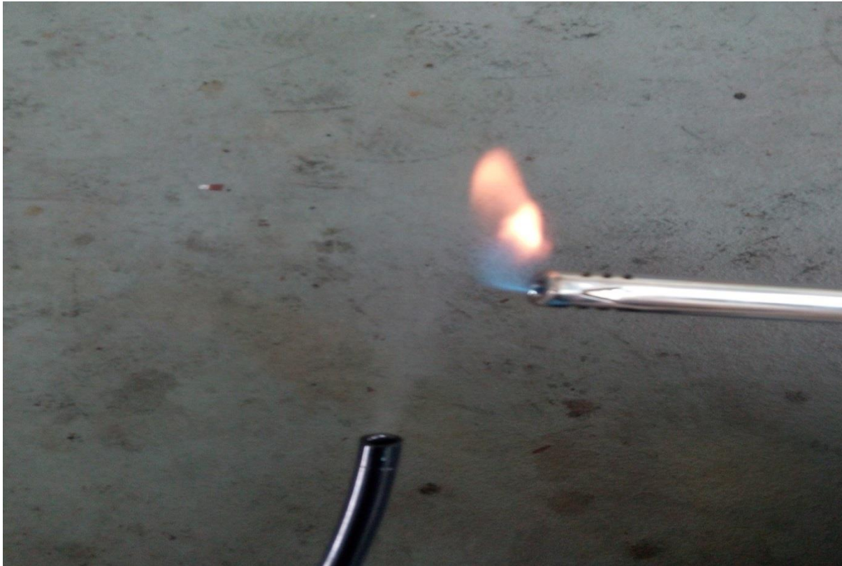
Figure 6-5c: The lighter after the syngas is passed on it (the syngas changes the colour of the flame as it is burning).
