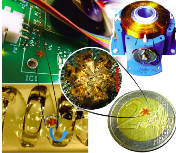
Figure 7.1. Soft grippers. Top Left: Image of a soft untethered gripper on a printed circuit board. Top Right: The electromagnetic setup consisting of six orthogonally-oriented electromagnetic coils. Center: Image of the closed gripper. Bottom Left: Video snapshot images of the gripper navigating through a tube with an inner diameter of 3.2 mm, a size smaller than most of the major vessels in the human body. Bottom Right: Image of the gripper on a 2€ coin. The scale bar is 0.4 mm.
