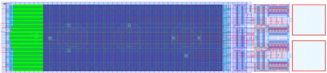
Figure 5.31: Layout of the MHUB Input and Output Pads.
