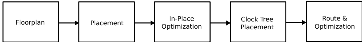
Figure A.4: Place and Route Flow.
