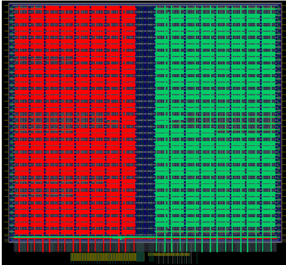
Figure 4.12: Layout View of the SA Multiply-Add Core with the Active Capacitors Highlighted. The main capacitor array for summing the partial product bits is highlighted in red, and the capacitor array for calibration and the additional add operation is in green.
