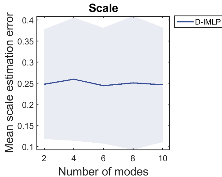
Figure 4.16: Scale experiment: errors in scale estimation using D-IMLP with increasing number of modes remain stable.
