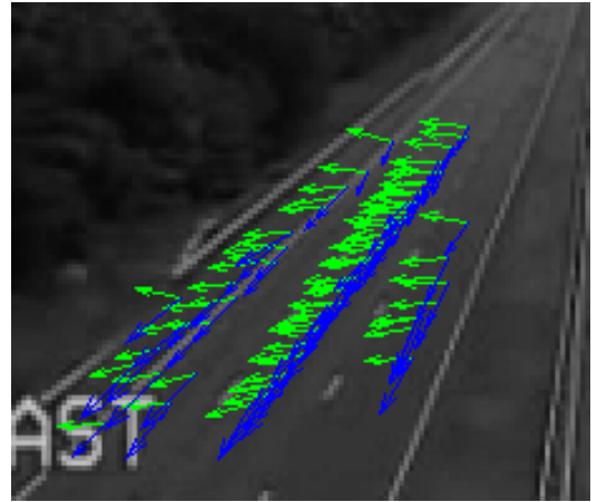
(b) The flow (blue) and transverse (green) vectors after 50 frames.
