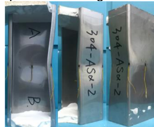
Figure 18 Distortional buckling of members with Section A
