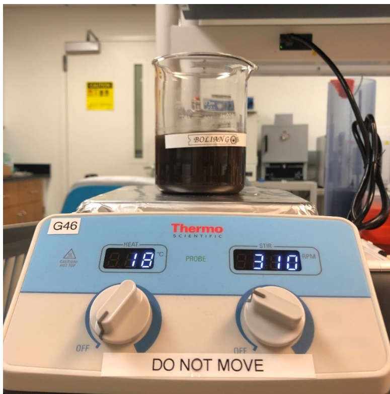
Figure 34 Mixing CNTs with polydopamine in Tris buffer
