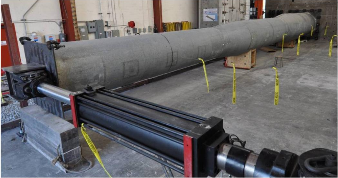
Figure 3.4 Test setup for full-scale test of 65 kW wind turbine tower (Sim et al. 2014).
