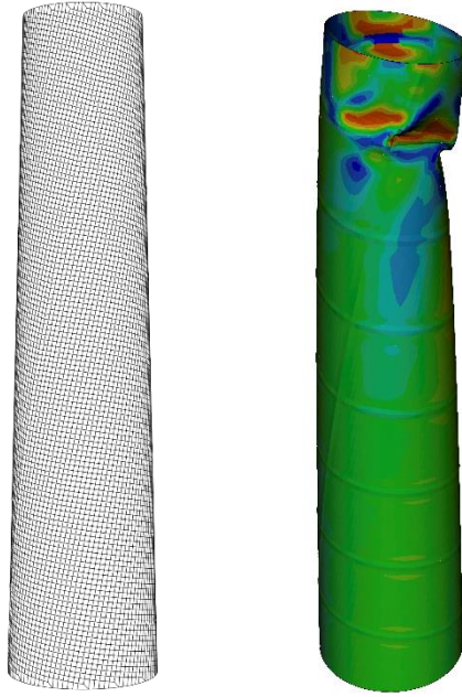
Figure 5.16 Full mesh of typical model of helically meshed tapered tube following the mesh guidance and the predicted collapse shape under bending.
