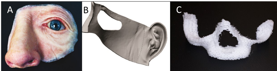
Figure 2-1. Examples of Rehabilitation, Reconstruction, and Regeneration. (A) Custom PDMS midfacial and ocular prosthesis. (B) Cutting and placement guides for auricular autogenous reconstruction. (C) 3D-printed maxilla, porous PCL scaffold.
