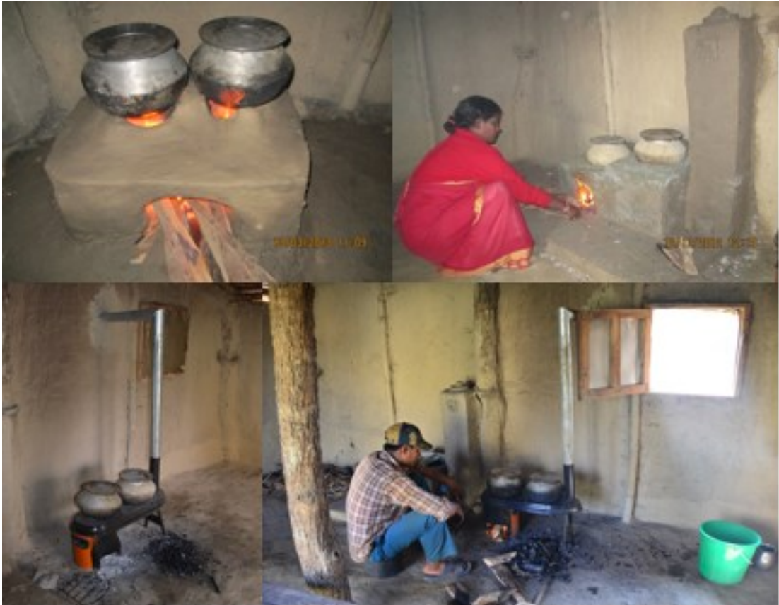
Figure 1: Stove types used for comparison. Top left: Traditional, open-design mud brick stove. Top right: Improved mud brick stove with chimney. Bottom left and right: Envirofit G3300/G3355 model stove (original model/manufacturer altered/NNIPS altered)
