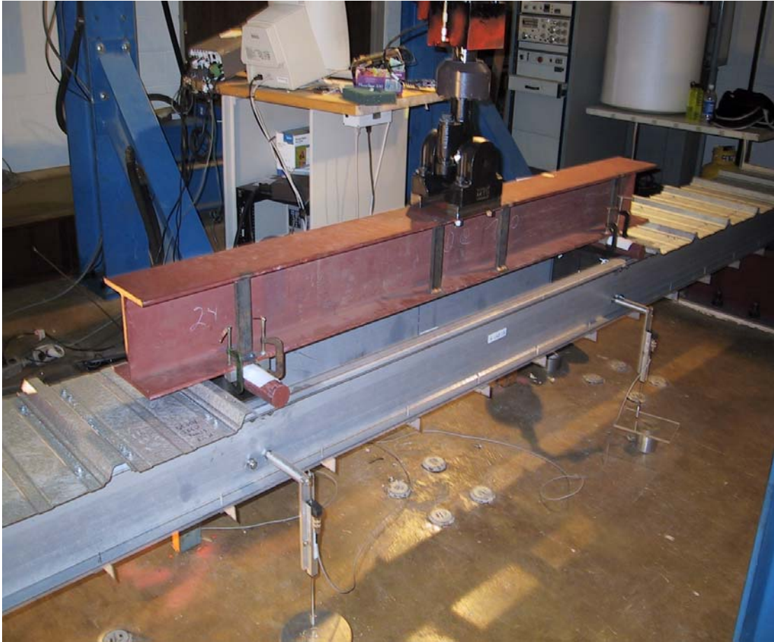
Figure 5 Yu & Schafer Test set-ups a) Local, b) Distortional
