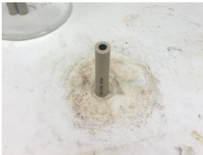
Figure 2.19 Photo of glassy carbon electrode with catalysts.
