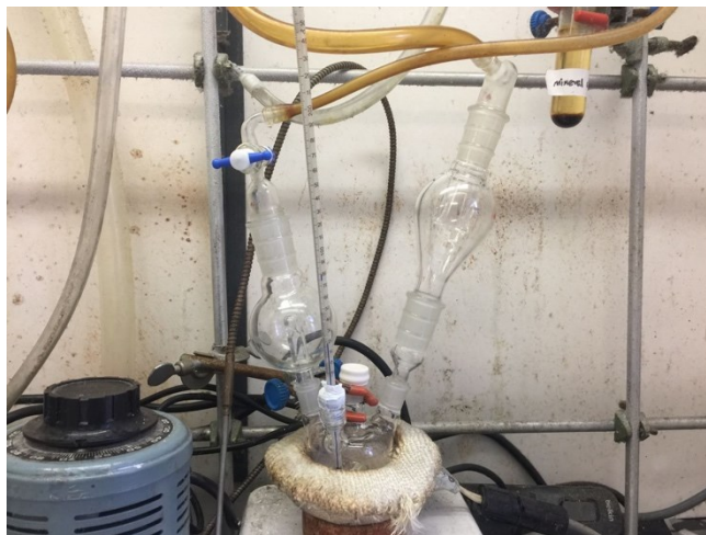
Figure 1.1 Photo of organic solvothermal synthesis experimental setup.
