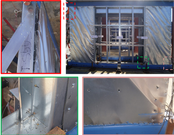
Figure 14: Photographs of SGGS-1 at end of monotonic test
