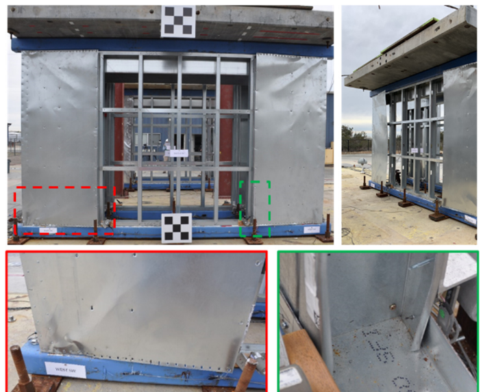
Figure 16: SGGS-2B specimen damage photographs after earthquake test EQ5
