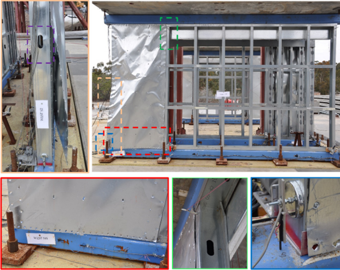
Figure 17: SGGG-1 specimen damage photographs after earthquake test EQ5
