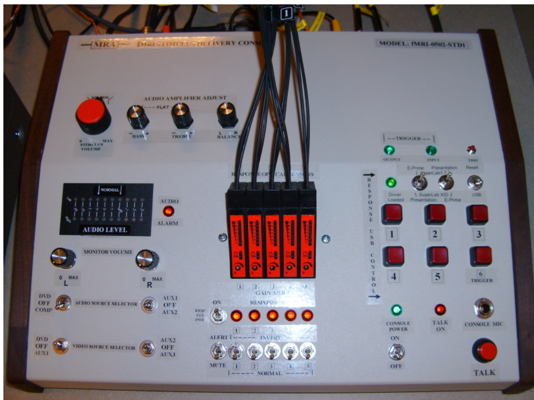
Figure 2.6: The Cedrus RB-830 response box used in our experiments. This device sends all fMRI-related signals over the serial port.
