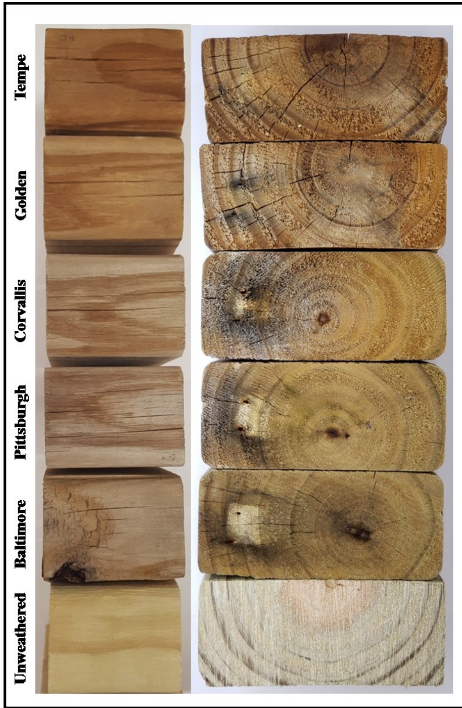
Figure 4-4: Images of pressure treated venti sized lumber before and after 18 months of outdoor weathering show from the top (top panel) and side profile (bottom panel).
