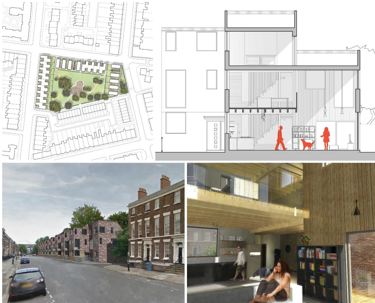
Figure 4. Site plan, section and perspectives. This project proposes two different house shells containing a staircase, kitchen and bathroom. Beyond these, it is up to the end-user how space is tailored to the needs of its inhabitants. This concept was explored by applying three different scenarios to each of the shells and examining how those family types could appropriate the space. By Matthew Kerrod.
