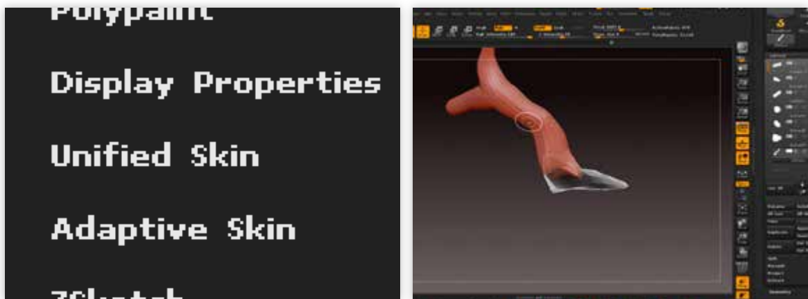
Figure 45 Adaptive skin (left image) was used to convert the ZSphere into a meshed surface (right image) for further modeling.
