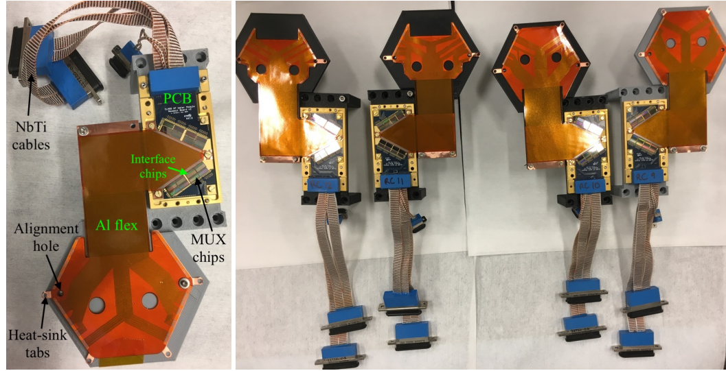
Figure A.3: Readout Circuit Assembly: While the feedhorn and detector wafer are being assembled as shown in Figure A.2, the readout circuits can be assembled simultaneously in a separate setup. As shown in the image on the left, first, a Au-plated copper structure that supports the readout package in the HF module is mounted on a 3D-printed jig. A PCB with twisted pairs of NbTi signal cables soldered onto it is bolted to the copper support. A Nb sheet (not shown here) is sandwiched between the PCB and the copper support for magnetic shielding. Then, the MUX and the interface (containing shunt resistors and Nyquist inductors) chips are glued onto the PCB with rubber cement. One end of the Al flex circuit is also bolted to the copper package as shown here. The jig is then moved to the wirebonder. A set of Al wirebonds are put down to electrically connect the Al traces to the signal cables through the interface and the MUX chips, and the vias on the PCB. The four MUX chips on each side of the readout package are also strung together through Al wirebonds to form a multiplexing column with 44 channels each. For a schematic of the wirebonds used to connect the different readout components, refer to Figure 3.6. The above readout package assembly is repeated for three more circuits as shown in the image on the right. While the Al flex circuit for the four readout packages are different, the assembly procedure is the same.
