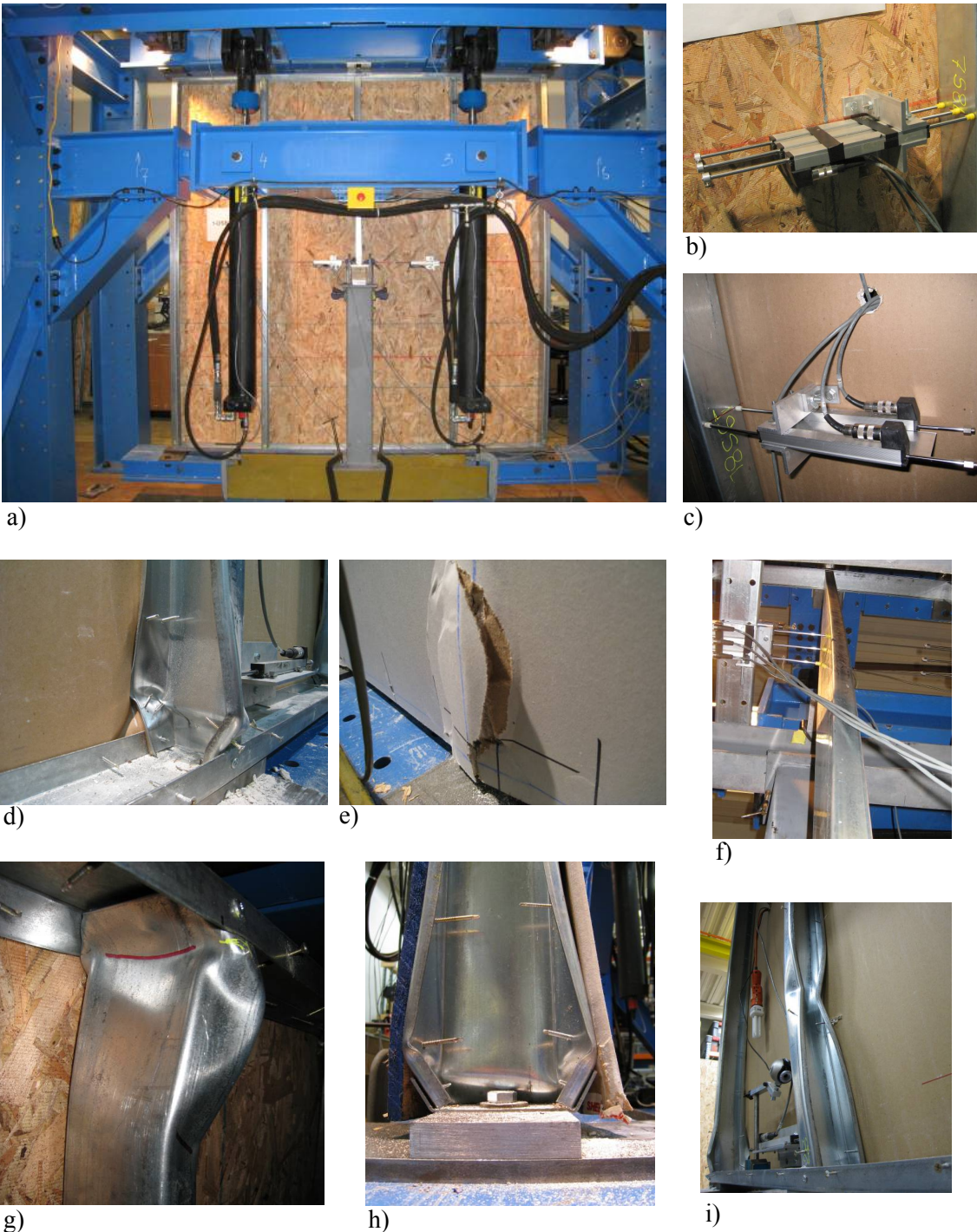
Figure 3 – Tests of sheathed cold-formed steel stud walls under compression: (a) side view of wall in MDOF testing rig before testing; (b) and (c) PT sensors for measuring stud deformations; (d) Gyp-Gyp wall opened after test to show local buckling at the ends; (e) local buckling tearing gypsum board; (f) flexural-torsional buckling of unsheathed Bare-Bare wall; local buckling (g) at the top of OSB-OSB wall, (h) at the bottom of OSB-Gyp wall, (i) followed by distortional buckling on Gyp-Gyp wall.
