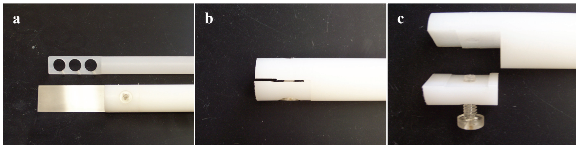
Figure 2-2: Redesigned coupon holders for the biofilm reactor, showing (a) the original triple coupon holder compared to the redesigned holder with a microscope slide in place, (b) side view of the redesigned holder clamping mechanism, (c) side detail, disassembled.
