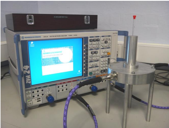
Fig. 1. Experimental setup showing VNA and the microwave resonant cavity with a sample in NMR tube.
