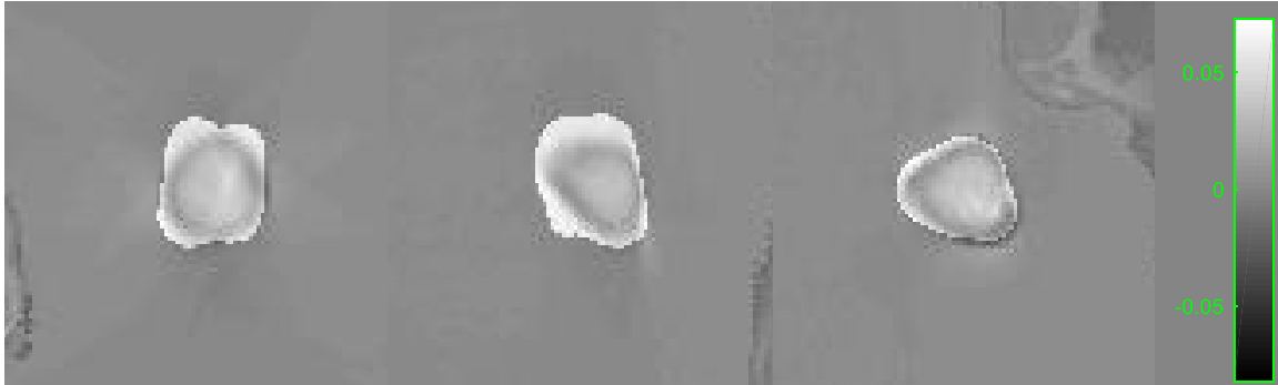
Figure 12: A magnified, cropped view of the difference image centered on the metal coil. The images demonstrate an acceptable approximation of the coil shape and size after segmentation in all three views.
