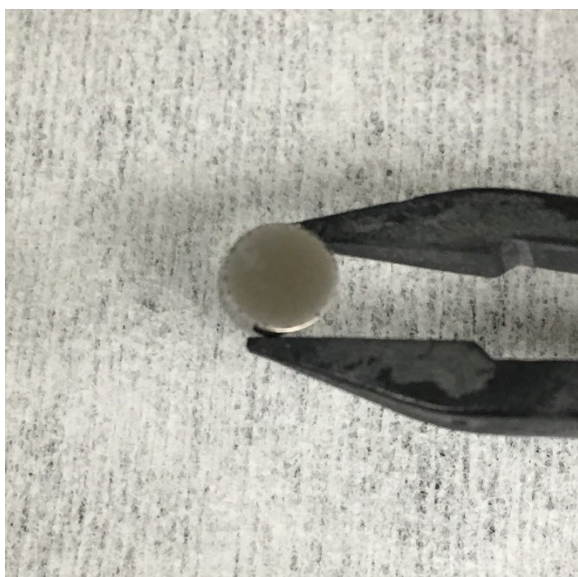
Figure 7. Pd thin film prepared by pulsed electrodeposition on a glassy carbon RDE
