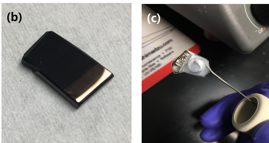
Figure 6. (a) Electrochemical cell setup for electrodeposition of Cu-Pd alloy (b) Cu-Pd alloy prepared by electrodeposition on a glassy carbon plate at -0.641 V vs. Hg/HgSO 4 for 600 s (c) Corrosion of Cu-Pd thin films after an electrochemical reduction reaction with high voltage applied
