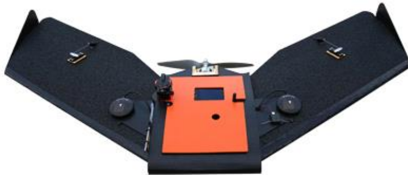
Figure 2-3: Tuffwing unmanned aerial vehicle flights. The orange panel can be removed to access the sensor payload.
