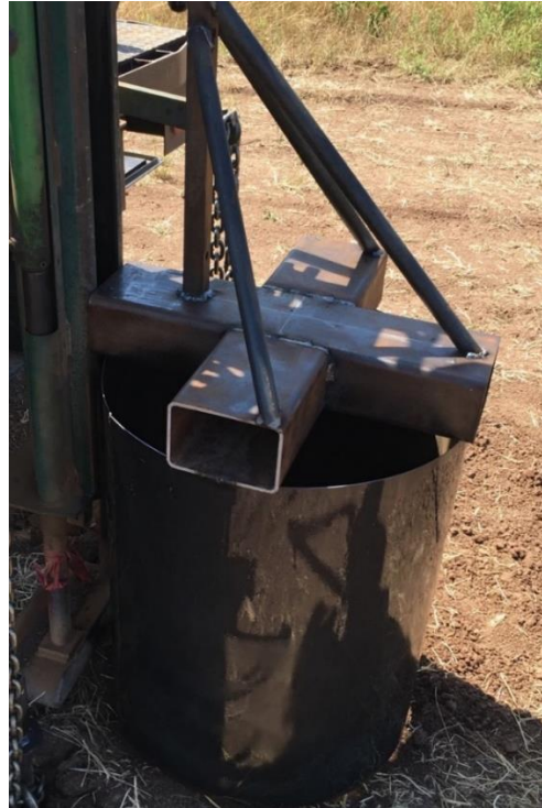
Figure 4-13: The annular core was constructed of 16 gauge steel, with 1 in cold rolled steel supports. It was designed to be attached to a Giddings probe.
