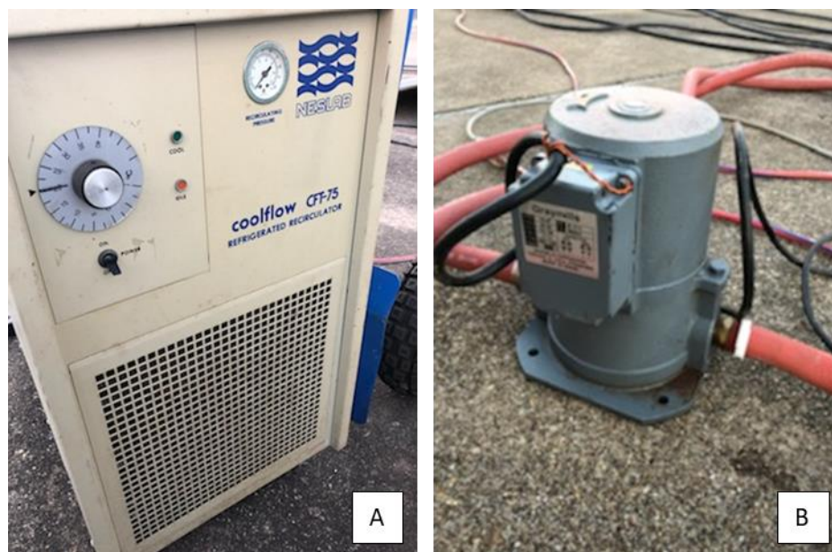
Figure 4-9: A) The Neslab CFT-75 water chiller was used to remove heat from the electromagnet oil bath. B) The oil pump was used to recirculate the oil to ensure that the electromagnet did not overheat.
