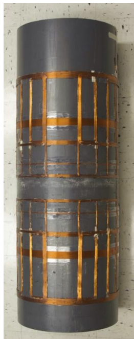
Figure 4-7: The gradient coils for the LF-MRI magnet. The z gradient coils were wound directly onto the plastic polyvinyl chloride (PVC) pipe, while the x and y gradient coils were constructed using a form and attached later. The gradient coils are located between the magnet and the radio frequency coil.
