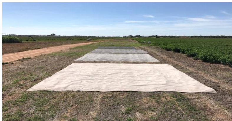
Figure 2-5: Aerial calibration tarps used in radiometric calibration of manned aircraft images
