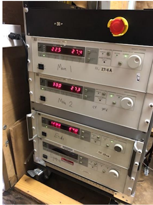
Figure 4-6: Three switching power supplies used for powering the magnetic field. Two were used for the main coil and one was used for the end correction coils.
