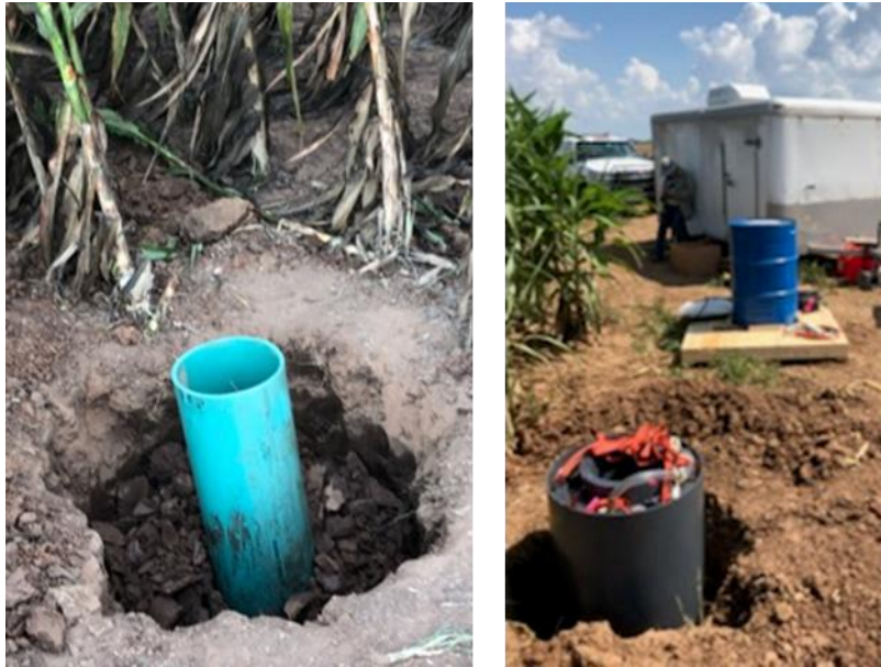
Figure 4-11: The LF-MRI electromagnet assembly is placed in the annular shaped hole around the green plastic polyvinyl chloride (PVC) pipe, which is centered around a sorghum plant.
