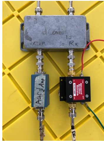
Figure 4-10: The combiner/splitter is used to drive the quadrature radio frequency coils.
