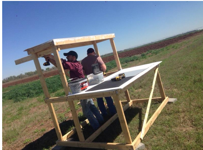
Figure 2-4: The ground control points were constructed with two levels, with radiometric targets placed on both the top and the bottom. The gps information was collected from the front corners of the lower deck.
