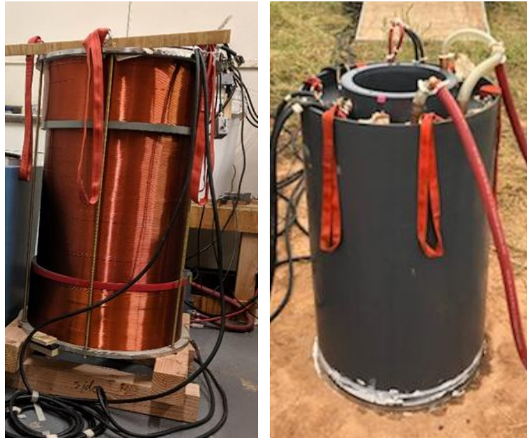
Figure 4-5: The magnet was constructed on a stainless-steel bobbin, wound with copper wire. The gray plastic polyvinyl chloride (PVC) housing holds in recirculating oil to cool the magnet.
