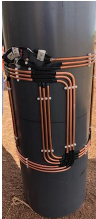
Figure 4-8: The radio frequency coil was constructed using a quadrature design with x and y direction saddle coils and was wound on 28.9 cm plastic polyvinyl chloride (PVC) pipe.
