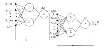
**Figure 4:** Module recurrent pi-sigma pipelined neural network architecture with *m* external inputs and second order pi-sigma units.
