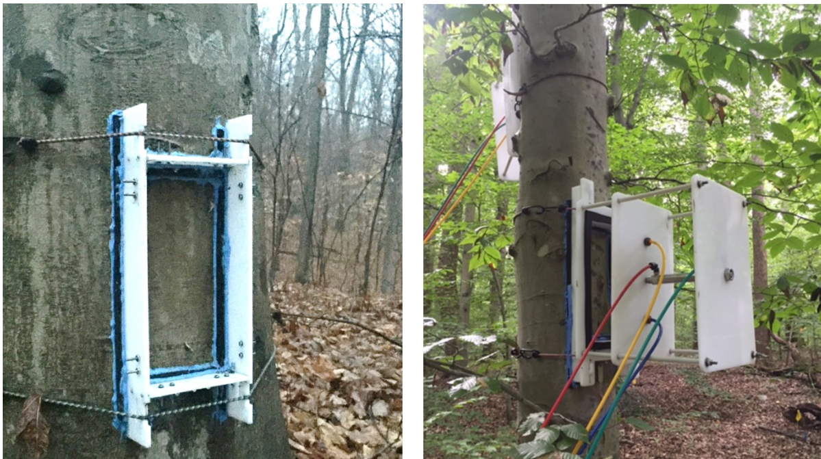
Figure 2-2: Example of the two types of flux chambers used in the study. Left: seventeen trees were fitted with manual chambers that remained in place and open between flux measurements over the course of a growing season (May-Sep). Fluxes were measured by securing a lid over the chamber and measuring concentrations for 5-10 min. Right: an automated version of the same chamber design.
