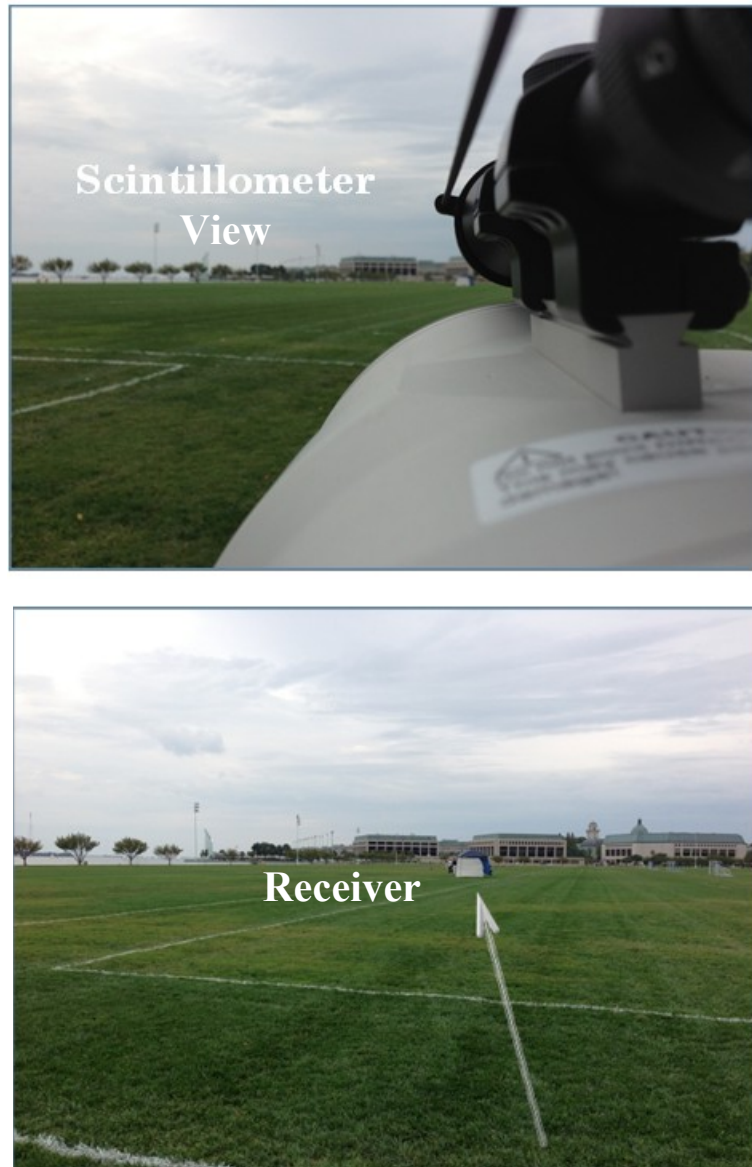
Figure 6.1 – USNA field tests, arrows show direction of laser beam propagation [7] – 180 m IR (1550 nm) laser beam propagation, scintillometer view is seen in top image and propagation path to the receiver in the bottom image. Note: The scintillometer was aligned along the beam path, but due to misalignment, good scintillometer data was not received for this case.
