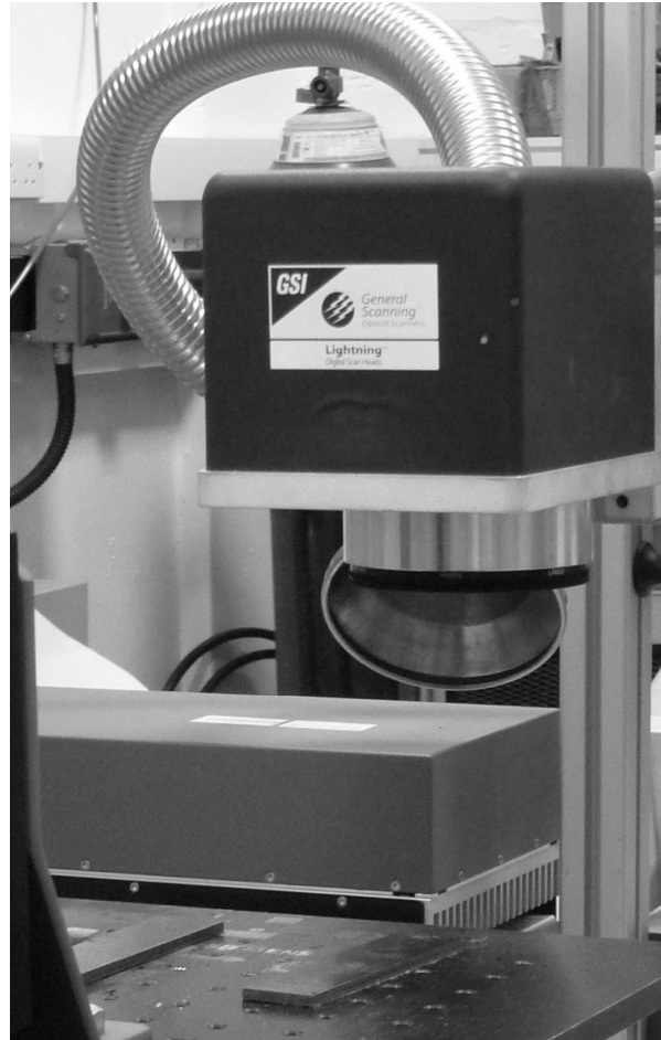
Figure 1: SPI Laser processing experimental set – SPI laser in background, GSI Scanning head in foreground.
