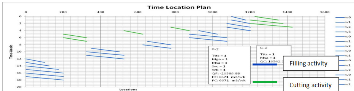
Fig. 7: Time location plan generated by the prototype model with option 4
