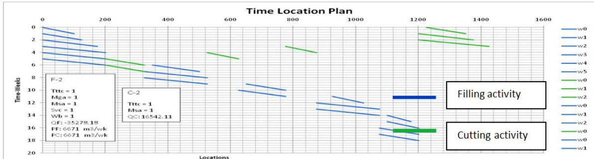
Fig. 6: Time-location plan generated by the prototype model with option 3
