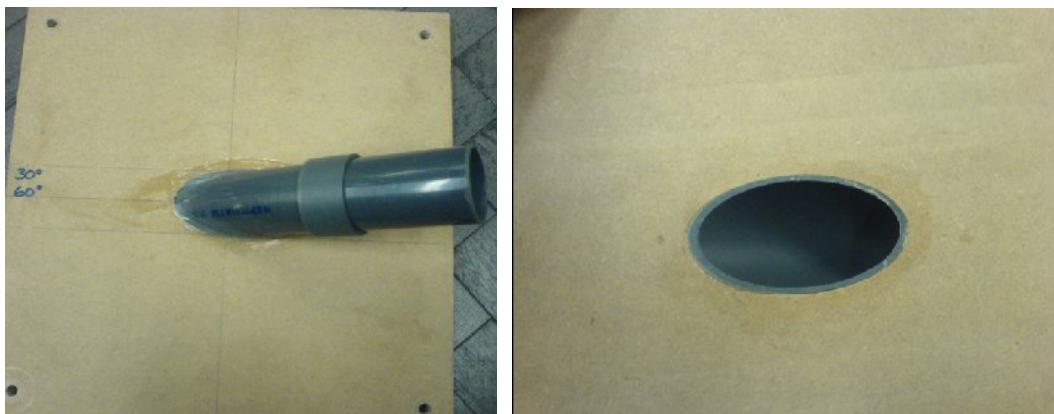
Figure 2.10: Oblique angled duct ( 60^\circ ) Front and Back View
