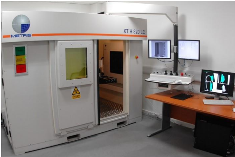
Figure 3-4 The (Nikon XT H 225/320 LC) micro X-ray Computed Tomography scanner, located at Warwick Manufacturing Group (WMG), used to scan the packed spheres sample.
