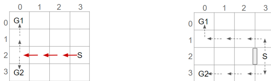
(a) The longest non-distinctive plan prefix from the start location (S), which is part of an optimal plan for the two goals (G1 and G2), is indicated by red arrows. The WCD for this environment is 3. (b) By preventing the human from performing a single action, the goal of the human can be determined from their first action, i.e., WCD = 0.
