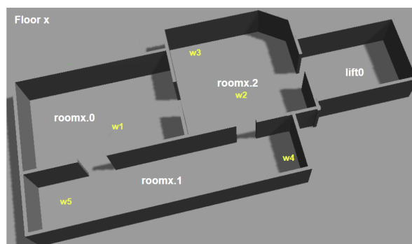
Figure 11. Gazebo simulated world used for the experiments. We use an extended version of the world originally created by Speck et al. [3]. Waypoints (e.g., w1) that are used during the different experiments have been indicated on the map. For all experiments there are also waypoints either side of doorways.
