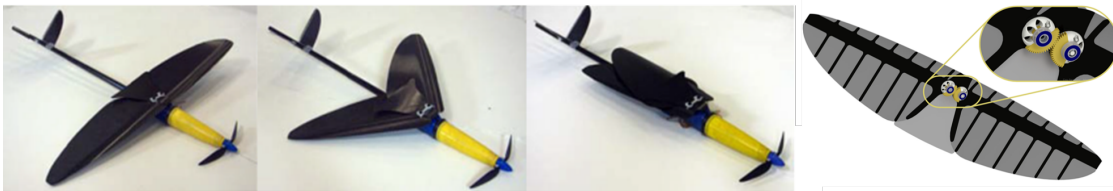
(b) Similar prototype vehicle: detail of folding wings (figure adapted from Ref. 11)
