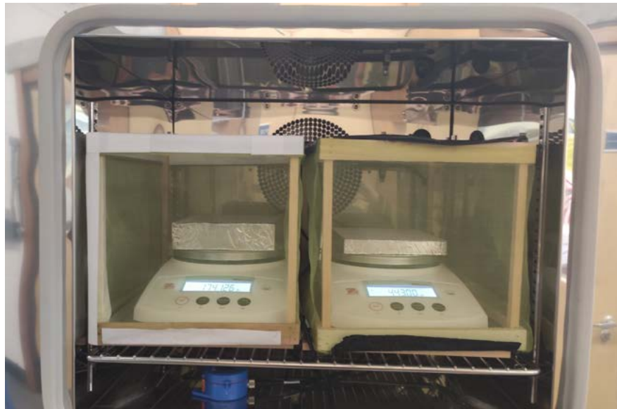
Fig. 3-6. Moisture buffering set up in the climatic chamber
