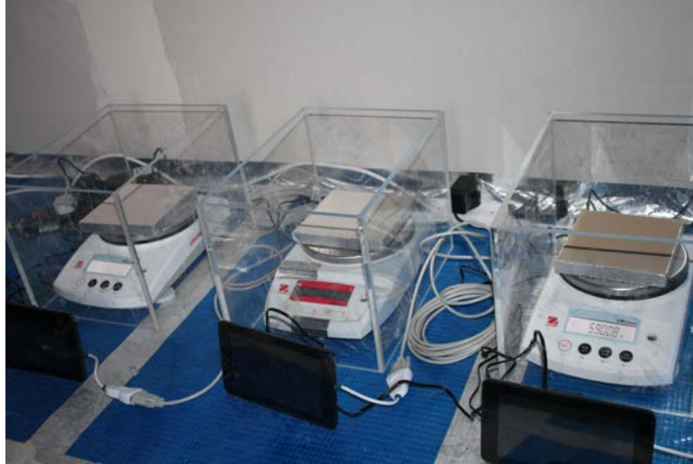
Fig. 4-32. Moisture buffering testing in the test cells at the BRP
