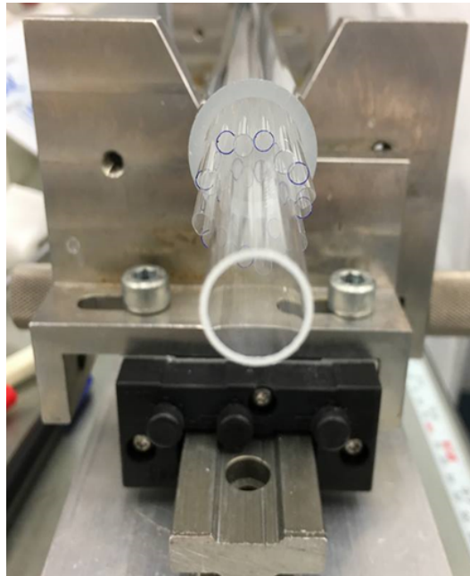
Figure 3.11 Image taken at the end of a stack session of a 6 ring hollow core fibre. The tubes marked with blue are the support tubes, and in between them there are 6 resonator tubes. In the middle there is a core support tube.
