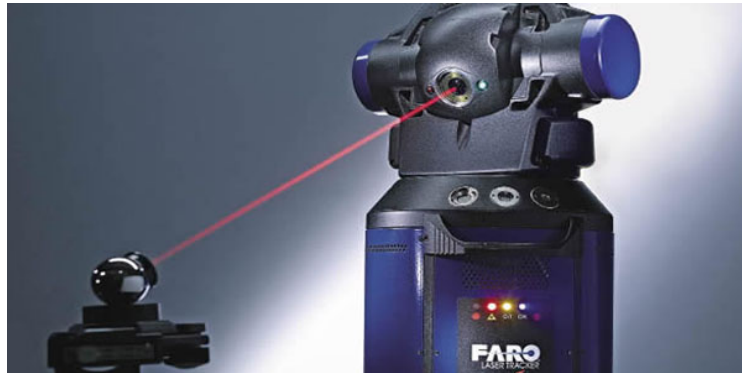
Figure 2.3 The FARO laser tracker following the SMR [34] .
