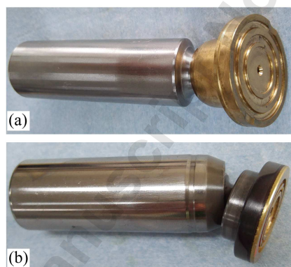
Fig. 13 Comparison between standard and “male” slippers: (a) standard “female” slipper; (b) “male” slipper
