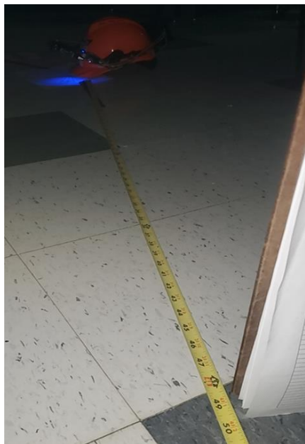
Figure 49.) LED and ToF Max Distance 49 inches (~1245mm).
