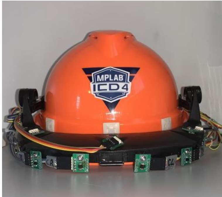
Figure 37.) Frontal View of Housing Unit, ToF Sensors and LEDs.
