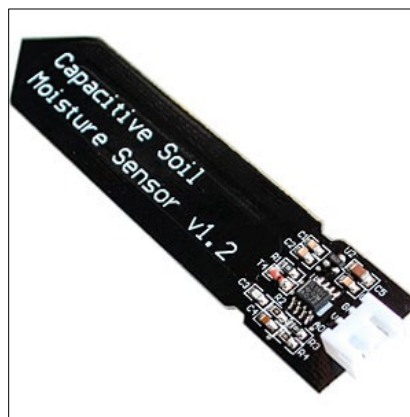
Figure 2: Analog Capacitive Soil Moisture Sensor. Image retrieved from https://www.reichelt.com/de/en/development-boards-soil-moisture-sensor-capacitive-analogue-debo-cap-sens-p223620.html?r=1 .
