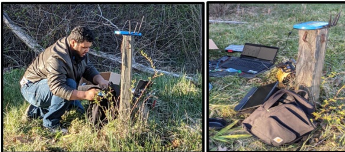
Figure 108: 3.3km Distance Testing Communication Setup.
