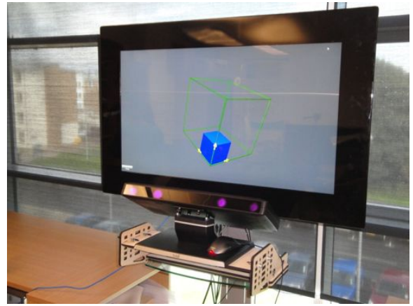
Figure 2: The Microsoft Pixsense mounted vertically and the Tobii X300 eye tracker placed on a custom laser cut wooden shelf.
