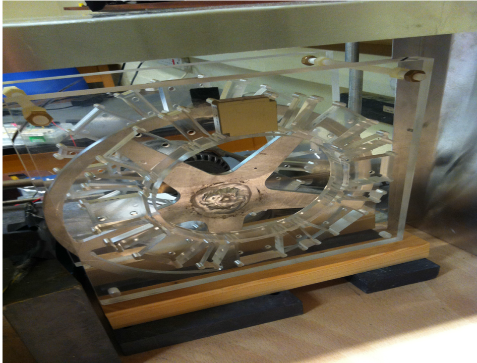
FIGURE 3.14: The image shows 1 magnet in the support structure in the foreground with the mini target wheel behind it. The blocks on the left of the image act to provide more stability when wheel is running. The motor is directly behind the wheel.
