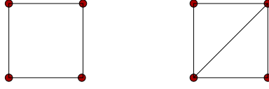
Figure 3.1: The square with one diagonal is rigid in 2D but flexible in 3D
