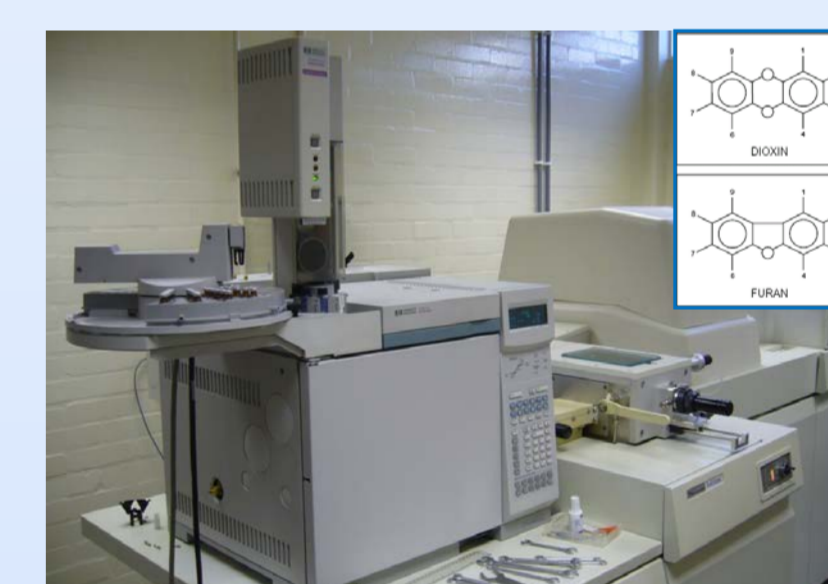
Fig. 6: HRGC-HRMS (HP 6890 Series / Autospec Ultima, Micromass) for the analysis of PCDD/Fs
