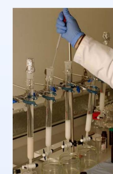
Fig. 4: GPC, one of the clean-up steps
