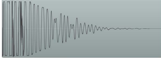
Figure 6: The clipped waveform of a tank projectile impact sound.
