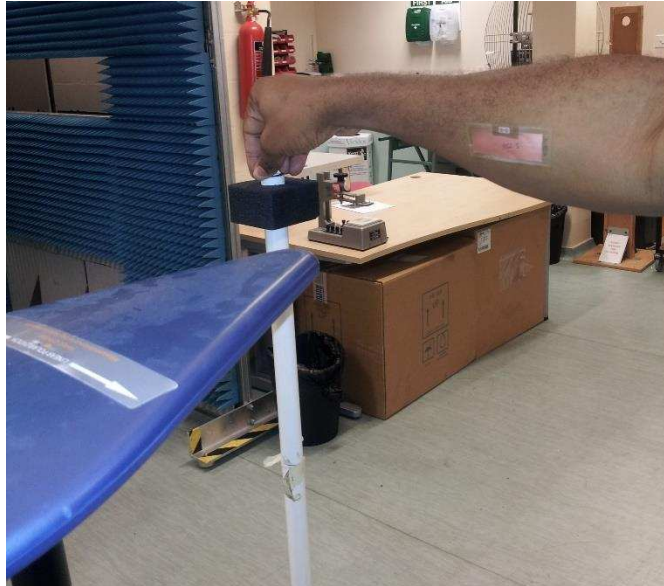
Fig. 3.16 Transfer Tattoo Tag performance measurement setup
