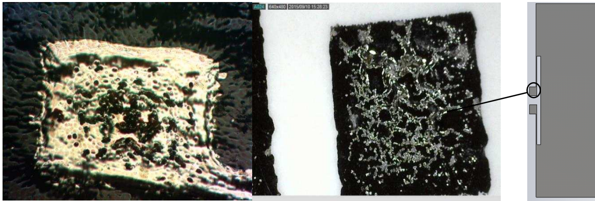
Fig. 5.6 Pinhole defects on the RFID tag port
