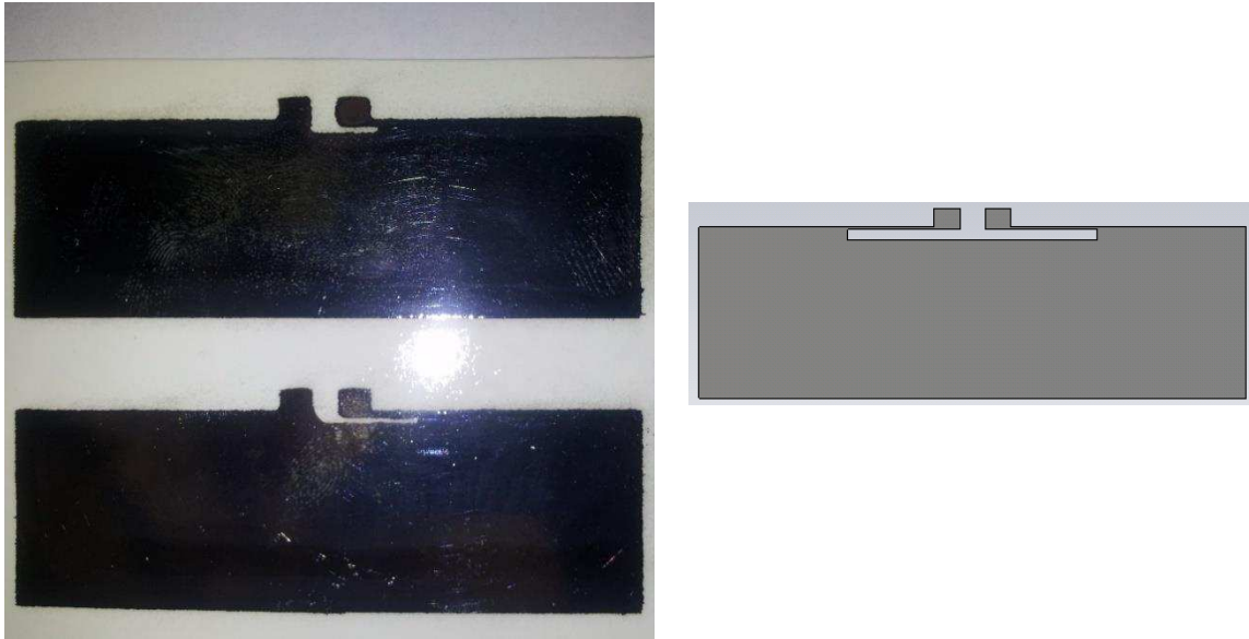
Fig. 4.5 Poorly Defined Pattern due to a Low Viscosity Ink
