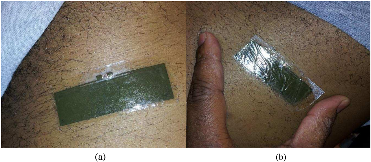
Fig. 5.27 Tattoo Tag mounted on Torso for Gym Test (a) Before Gym (b) After Gym
