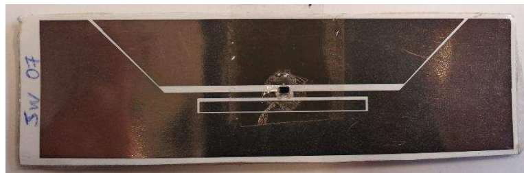
Fig. 6.10 Inkjet printed Tag using conductive ink
